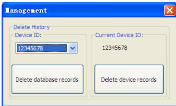
Click “Delete database records” button to delete the history data on the PC. The user should disconnect the device from the PC to stop the data transfer before they click “Delete database records” button.
