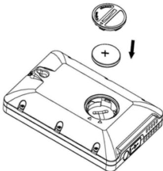
1). First use a large coin to open the battery cover at the back of the unit.
